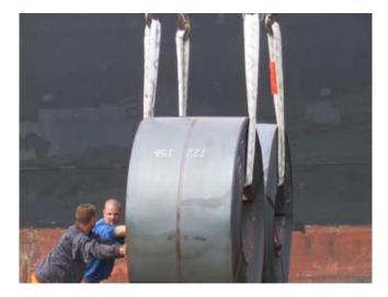
The slings are also soft, thus reduce the chance of damaging your load. The lower weight, even compared to polyester or aramids, enables easier handling and presents less danger to the crew handling them. There are fewer back injuries, for example. And in contrast to steel wire, which can fray and leave sharp edges, slings with Dyneema® have a very smooth surface.
