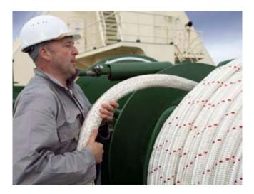
Mooring lines made with Dyneema® have shown lifetimes of over 10 years on frequently moored vessels, thus demonstrating the great possibilities of using Dyneema® fiber in this application.
