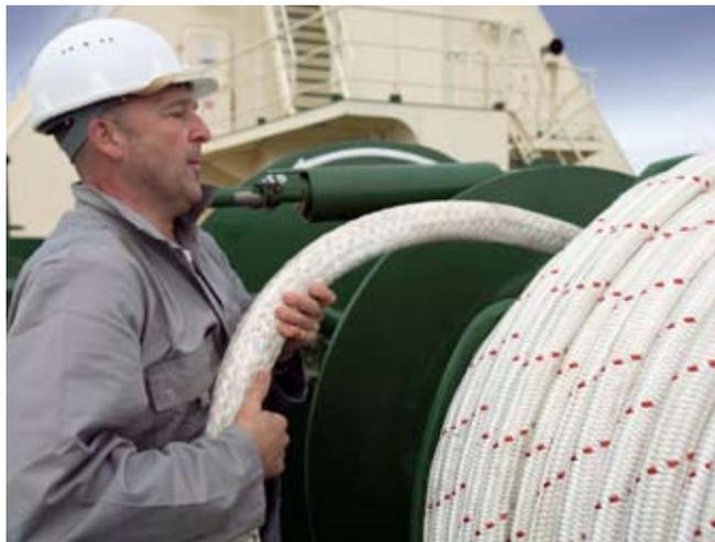
Mooring lines made with Dyneema® have shown lifetimes of over 10 years on frequently moored vessels, thus demonstrating the great possibilities of using Dyneema® fiber in this application.
