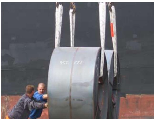
The slings are also soft, thus reduce the chance of damaging your load. The lower weight, even compared to polyester or aramids, enables easier handling and presents less danger to the crew handling them. There are fewer back injuries, for example. And in contrast to steel wire,
