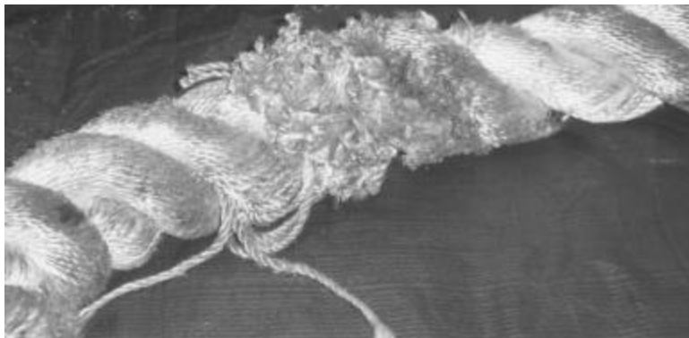
Figure D-008 Localized External Abrasion
