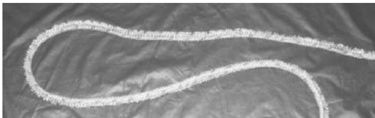
Figure D-005 Uniform Surface Abrasion (Tree limb bull line)
