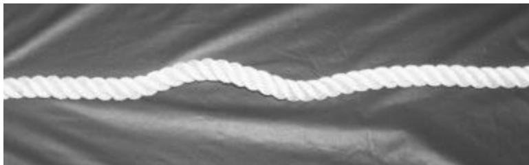
Figure D-024 Corkscrew Due to Twist
