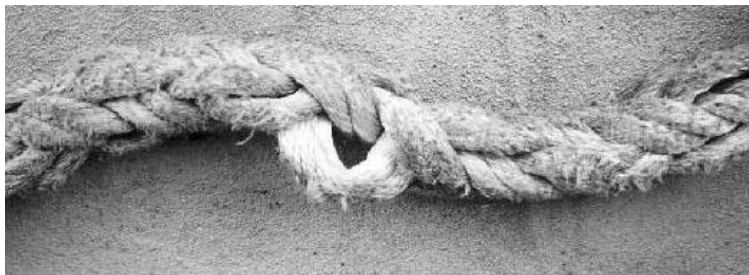
Figure D-013 Pulled Strand in 8 Strand Rope
