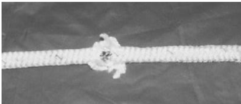
Figure D-012 Cut in Jacket Exposing Core
