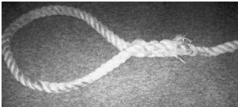
Figure D-018 3-Strand Splice of Poor Quality
